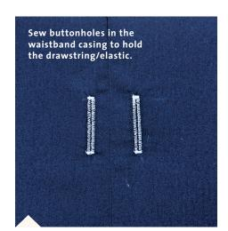
MAKE BUTTONHOLES IN THE CASING AREA. Centered at center front, fuse a 3-inch by 1-inch scrap of interfacing with its upper long edge parallel to and 1½ inches below the raw waist edge. Stitch a 3/4-inch-long vertical buttonhole on each side of the centerfront seam, with the buttonhole's top 13/4 inches from the waist edge. Cut the buttonholes open.
